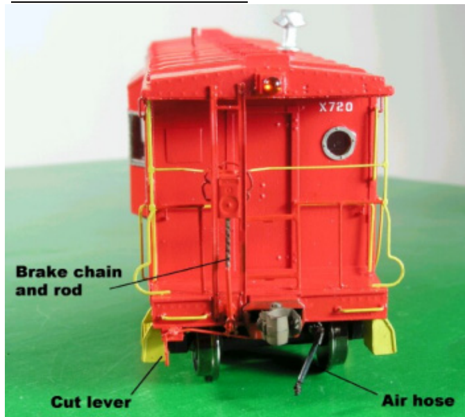
Photo 25a. Re-built end details.
