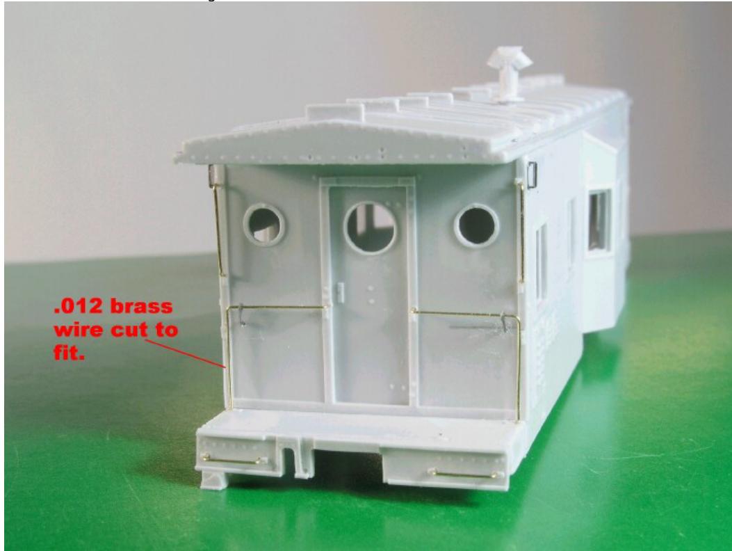
Photo 8. Install end corner grabs.
