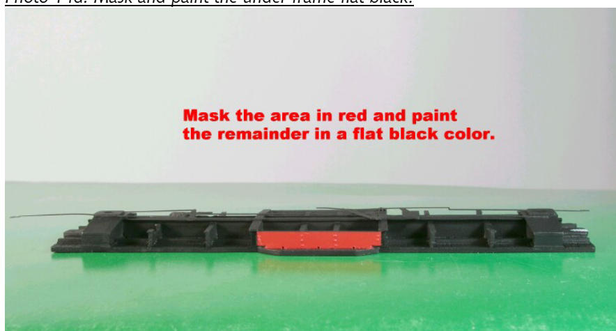
Photo 14d. Mask and paint the under frame flat black.
